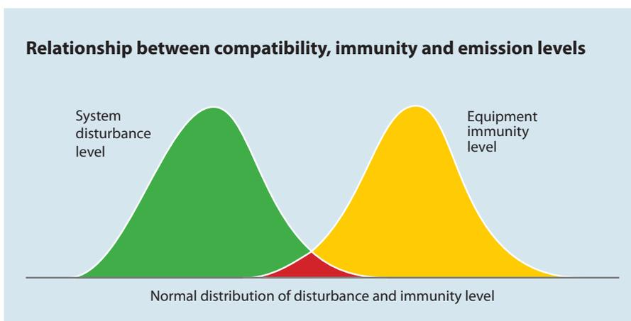
*A satisfactory operating production system is obtained when each installed equipment has an immunity that's higher than the total allowed grid distortion. For EN 61000-2-4 the immunity level is a minimum of 10% where as the planned highest distortion level is 5 or 8% depending on the installation. This leaves very few parts (red scattered) of the installation with temporary problems.*
