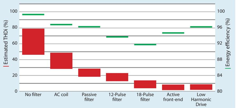
A comparison between different harmonic mitigation principles shows that low harmonic distortion is followed by low energy efficiency – except for active filtering, where the efficiency is relatively good.
