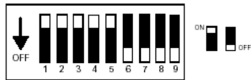
9600 Baud Rate and No Parity Switch Settings
