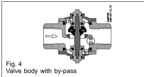
Valves of this type operate with significantly longer time constants than AVTA valves where the sensor is located at the point at which the temperature is to be regulated. FJVA is mainly used in systems where large and sudden load changes do not occur.
