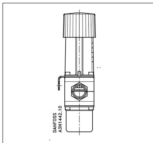
The valves can be installed in any position. An arrow on the valve body indicates the direction of flow.
